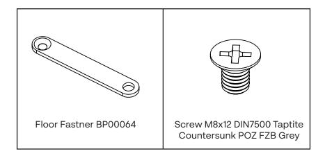
Note: Bolts for the floor bolting is not included. The hole in the floor fastner is fitted for using a M10 bolt. Diameter of the hole is 11mm.
