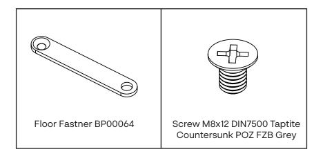
Note: Bolts for the floor bolting is not included. The hole in the floor fastner is fitted for using a M10 bolt. Diameter of the hole is 11mm.
