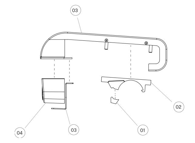
01. Bracket Clip. Attaches the bracket to the beam with M8 screws.
